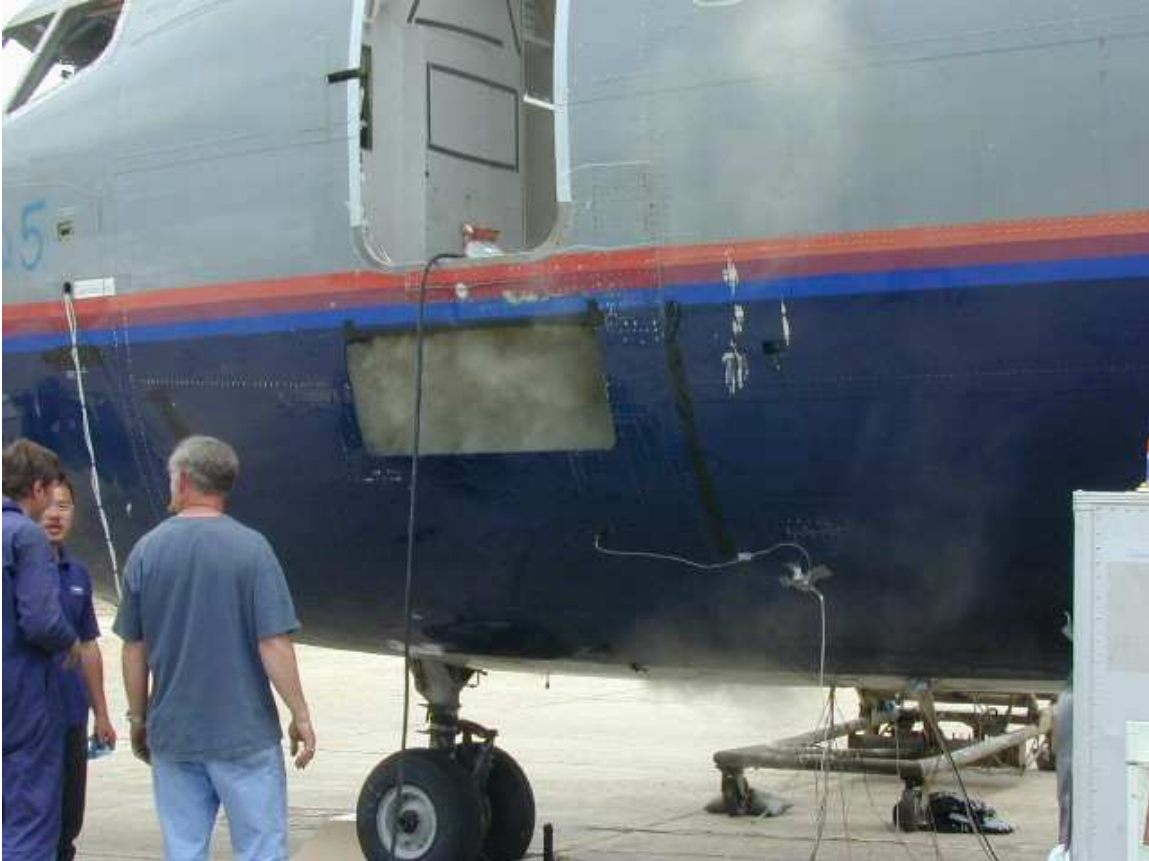
FIGURE 2 - PYROGEN AEROSOL DISCHARGE IN THE AIRCRAFT'S ELECTRONIC EQUIPMENT BAY
